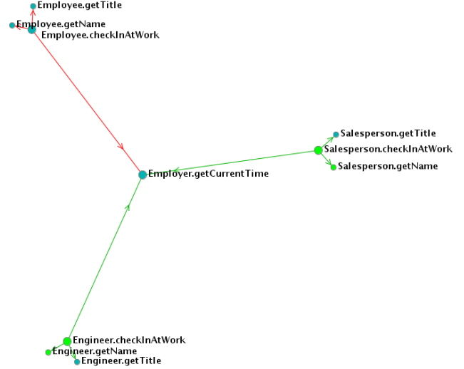
Figure 1. A ‘pull-up method’ refactoring removes 6 dependencies (green) and adds 3 (red), which improves the software structure
